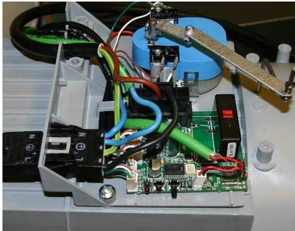
Figure 6 – Picture of controller card with cabling for a 1-relay version
